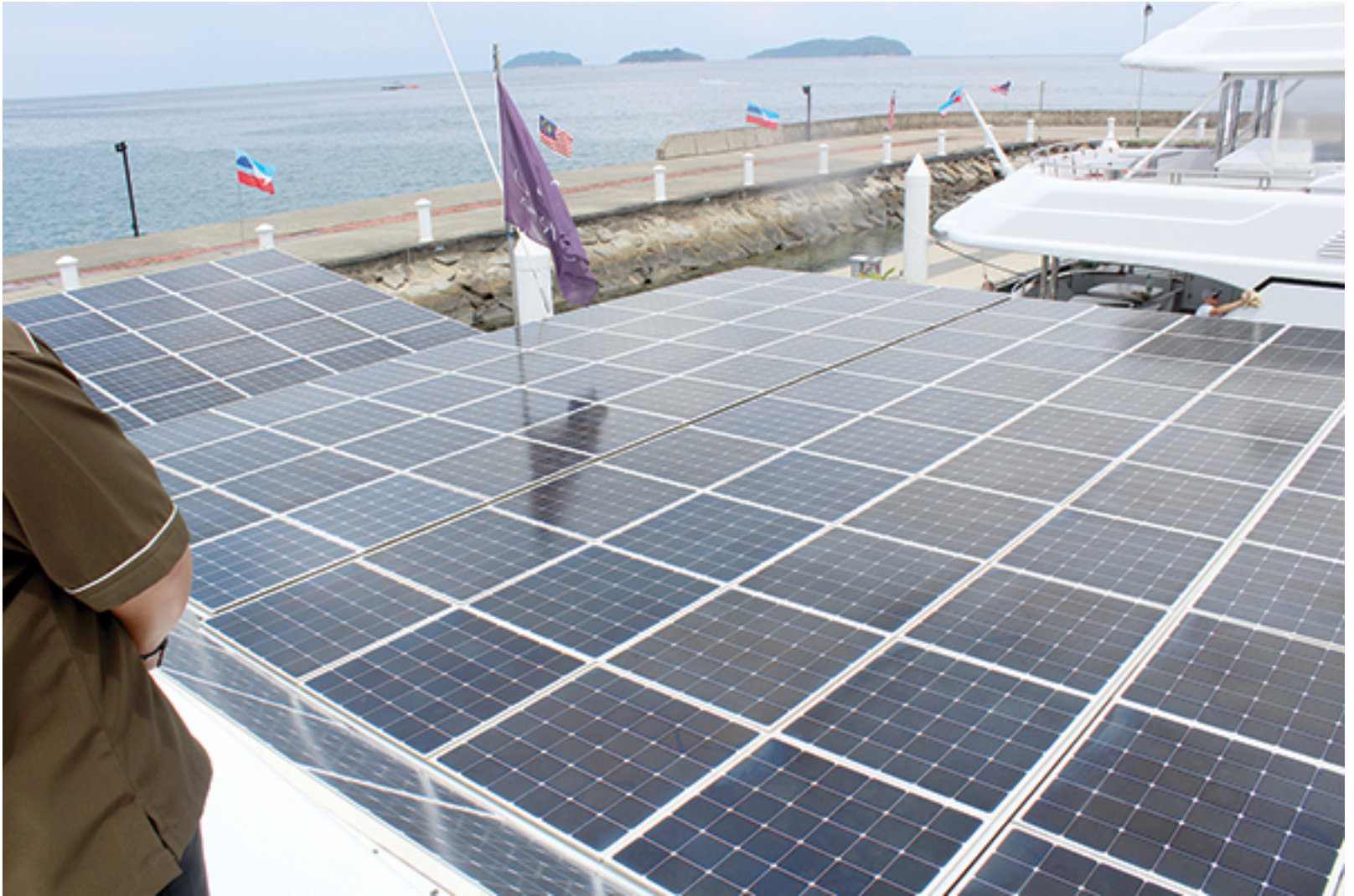
Part of the 512sq metres of solar panels which produce 67pc of electricity.
